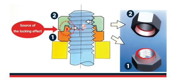
The vibration testing is based on the National Aerospace Standard (NAS 3350) which demonstrates the overwhelming superiority of the locking effect when compared with other products under identical conditions.
